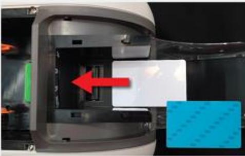
Remove the 3M peel off film on both sides of the clean card and put it into card hopper.
