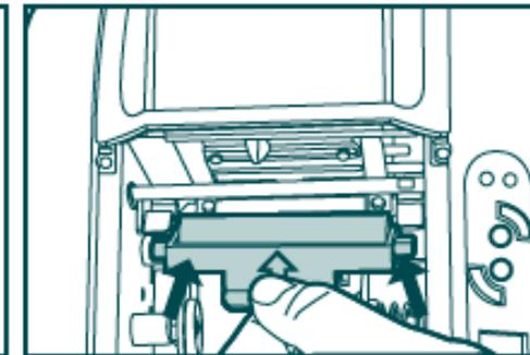
Place dust arrester back to the printer
