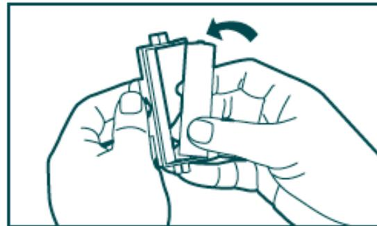
Assembly the roller and dust arrester
