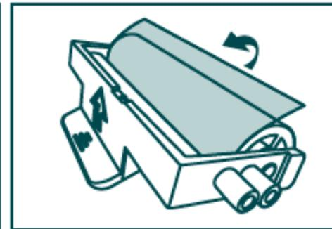
Remove adhesive film protection from cleaning roller
