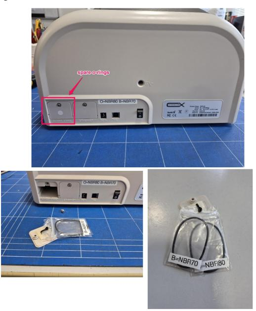
There you will find two bags labeled "B=NBR..." and "O=NBR...". These are the O-rings for the orange and blue sides, respectively. Further explanations can be found in the rest of the instructions.
